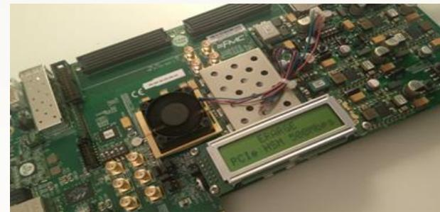
*Prigm©, Hardware Security Module with very high throughput (e.g. up to 1 Gbit/s TRNG), EAL4+ soon*
