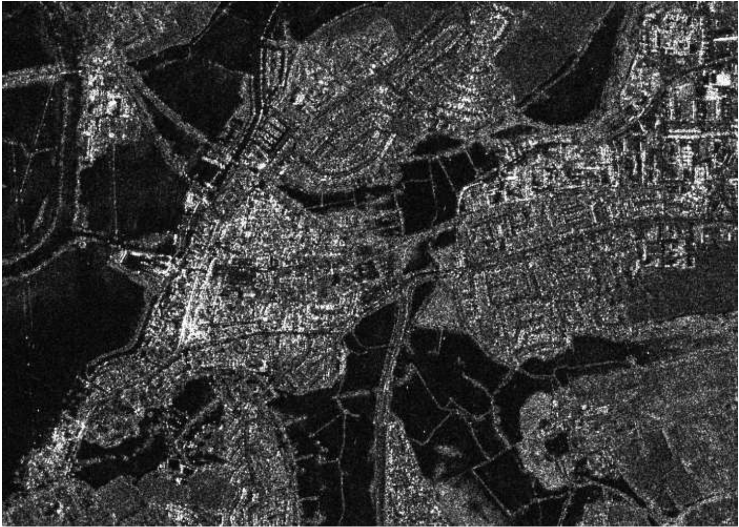
TerraSAR-X image of Tewkesbury flooding on 25 th July 2007 showing urban areas (3m resolution, dark areas are water).
