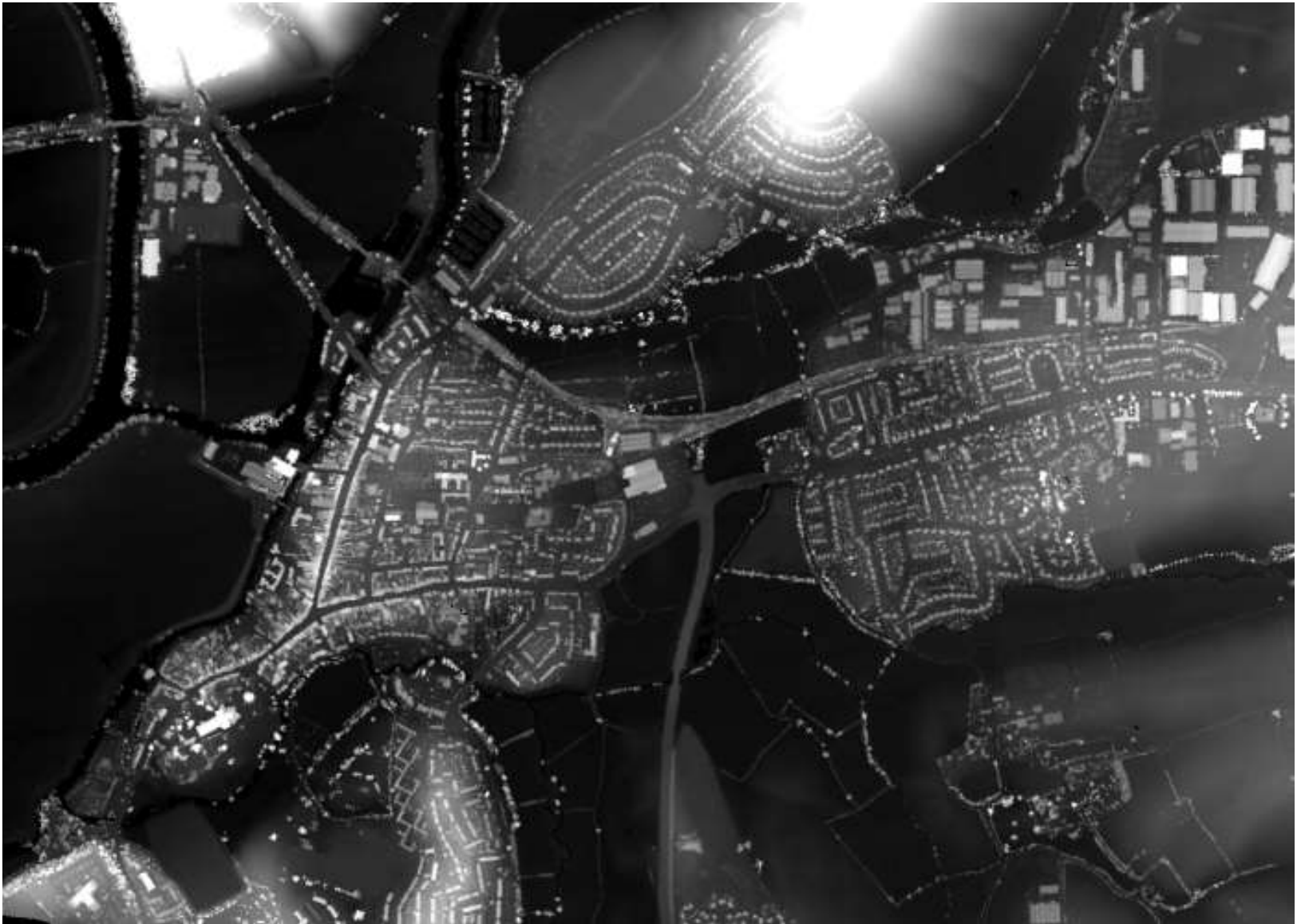
LiDAR DSM of Tewkesbury (2m resolution).
