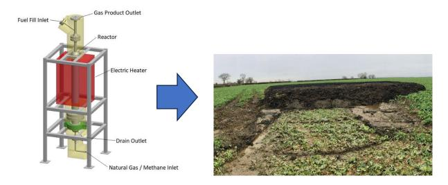
Methane cracking pilot plant which will produce graphitic carbon and mixed with manure to determine its suitability to establish crops
