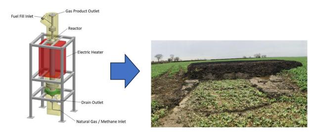
Methane cracking pilot plant which will produce graphitic carbon and mixed with manure to determine its suitability to establish crops
