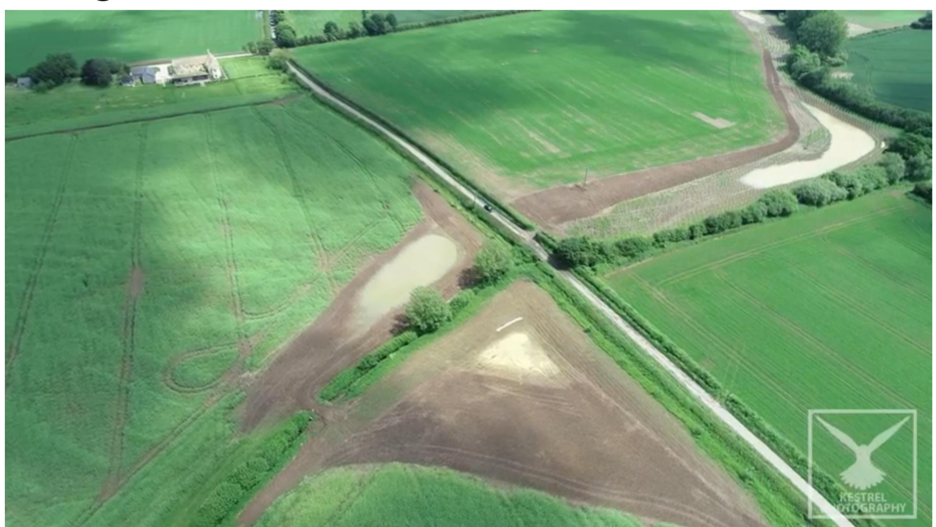
Left: Field-corner storage bunds partly filled after an intensive rainfall event in May 2018 (Image by Kestrel Photography)
