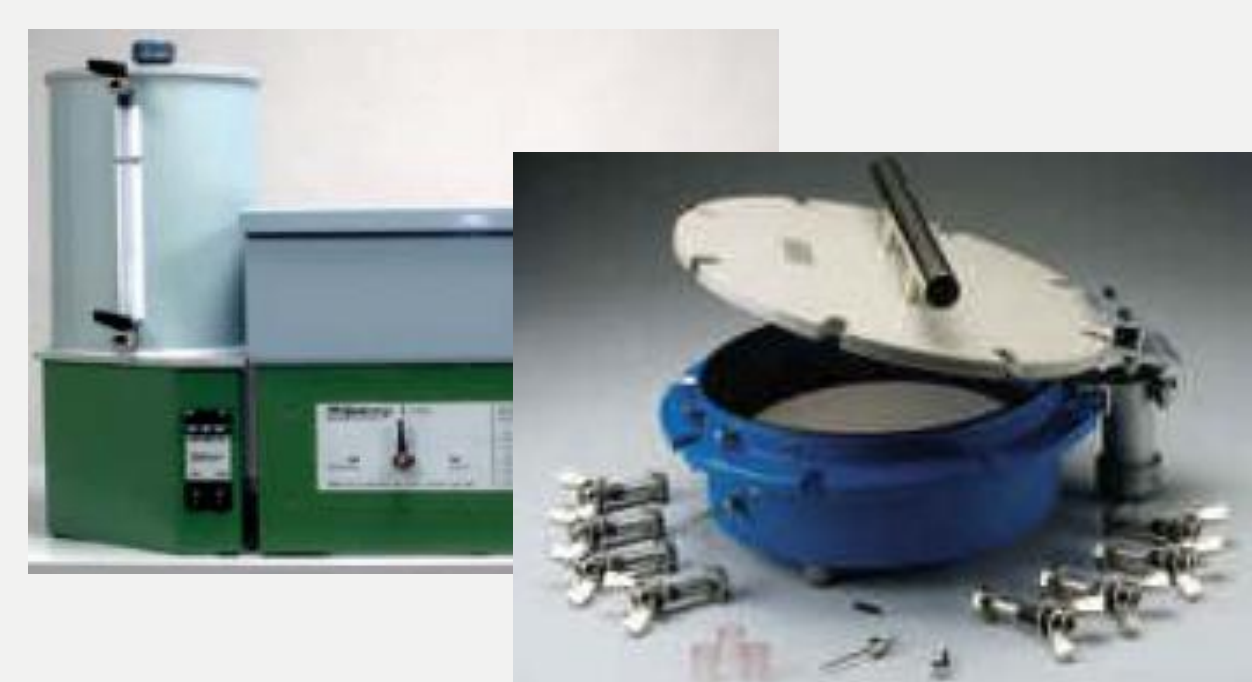
Soil moisture retention by sand/kaolin tables and pressure vessels
