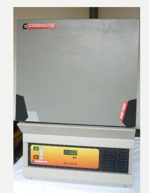
Soil organic matter by loss on ignition
