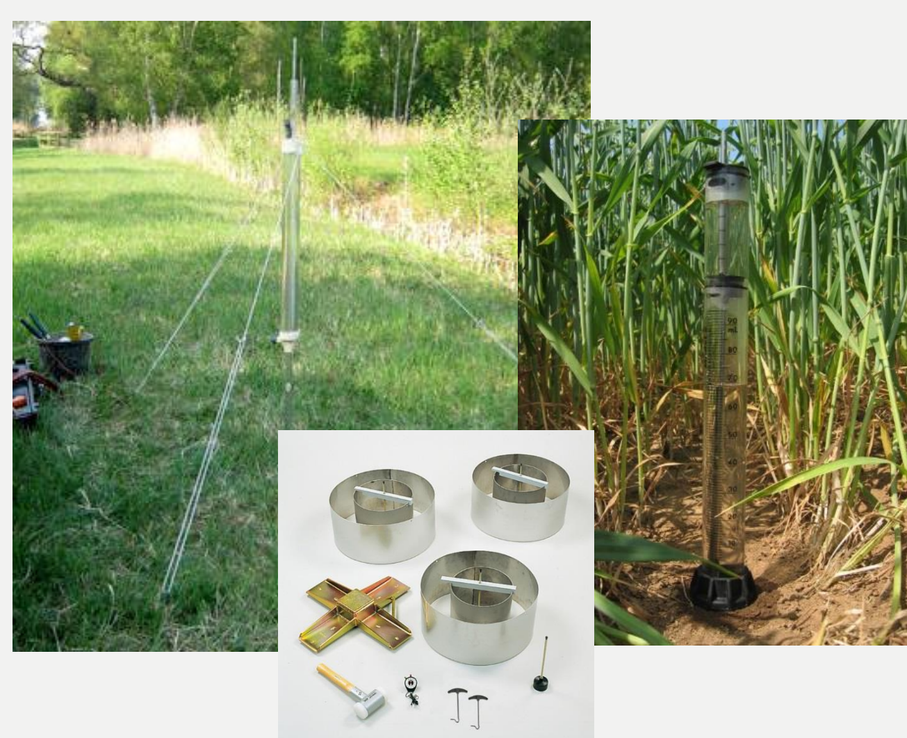
Soil hydraulic conductivity by Guelph permeameter, infiltration rate by double ring and/or mini disk infiltrometer
