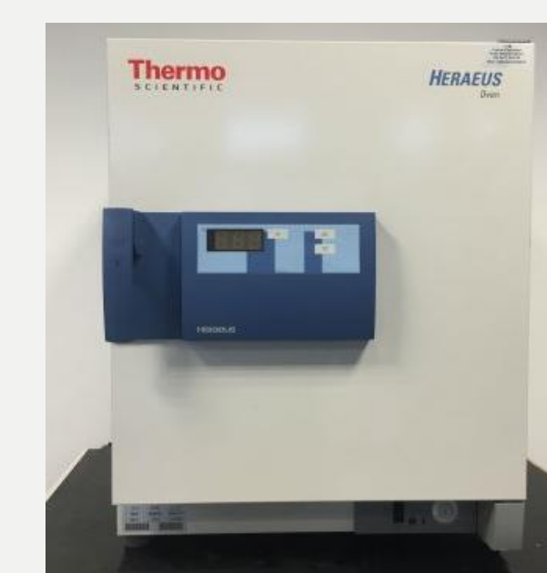
Soil moisture and bulk density by oven drying
