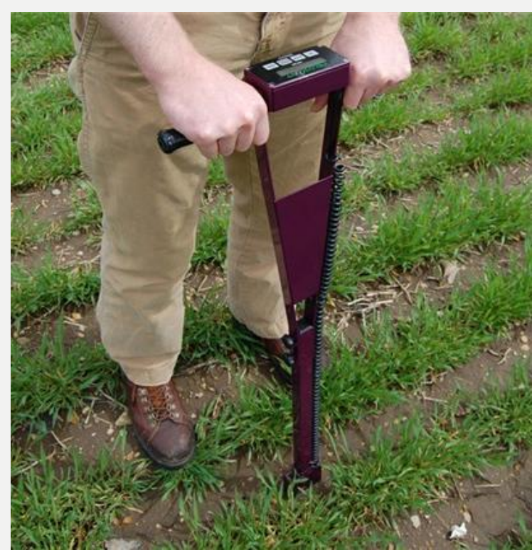
Surface soil moisture by roving TDR probe
