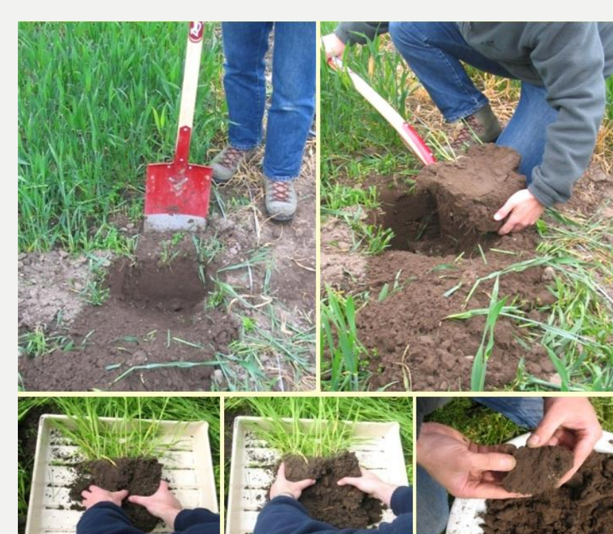
Visual Evaluation of Soil Structure; photo: SRUC
