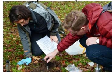
Citizen scientist also collect samples for further analysis in the laboratory, including: LOI, total C, soil colour and texture, water extractable carbon (UV-Vis, DOC) and water holding capacity. SUCTION RATE 1cm mini disk infiltrometer or soil compaction with pocket penetrometer.
