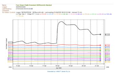
Sentek Drill & Drop 120cm soil moisture profile probe (Volumetric Water Content every 10cm) + Raingauge w telemetry (from www.soilmoisturesense.com/)
