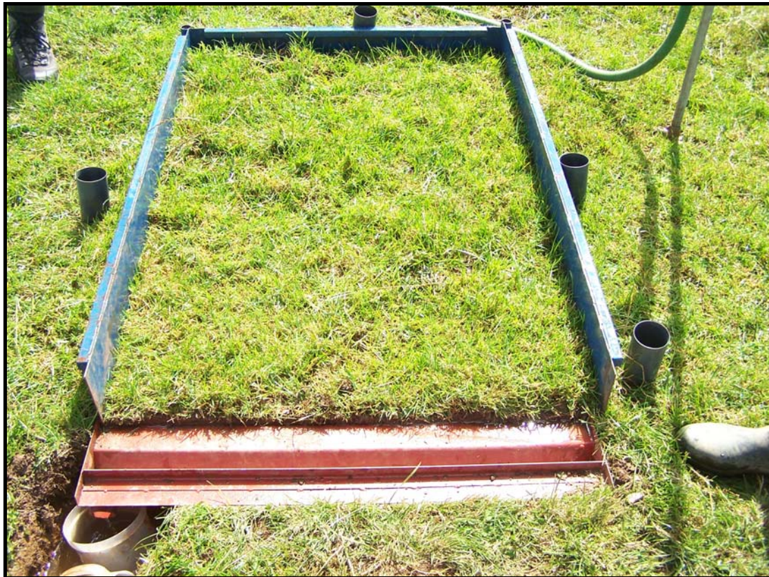
Figure 3: Rainfall simulation in progress. Photograph shows irrigation plot (blue) with rainfall cups measuring rainfall volume, tray collecting down-gradient surface runoff (red) and collection of runoff waters (bottom left).
