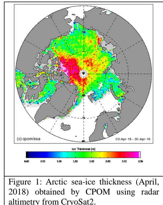
Figure 1: Arctic sea-ice thickness (April, 2018) obtained by CPOM using radar altimetry from CryoSat2.
