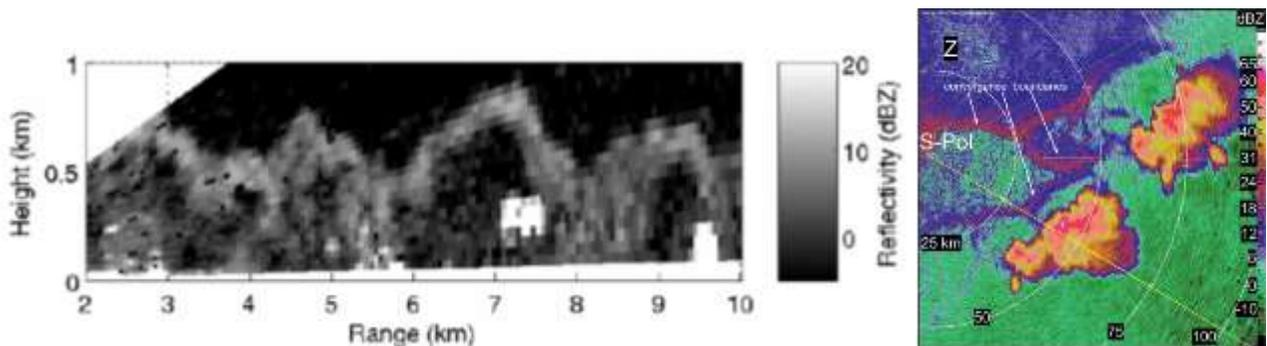
*Left: Signatures of sharp humidity gradients are detected in a vertical radar scan, indicating rising thermals along the edges of clouds. We can see that individual cells are 2 km apart (Bennet et al. 2006).*
