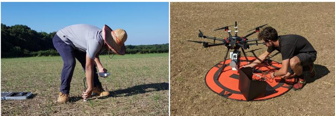
Figure 1. Field measurement scenes: moisture sampling (left); UAV-borne hyperspectral sensor (right).
