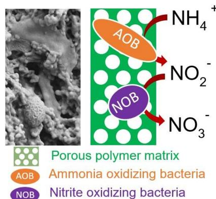
Already at the University of Surrey, our team has devised a biocoating containing metabolically-active *E. coli* bacteria as a model organism. More recently, we added nitrifying bacteria to a biocoating and successfully removed ammonium from water in a bioreactor.
