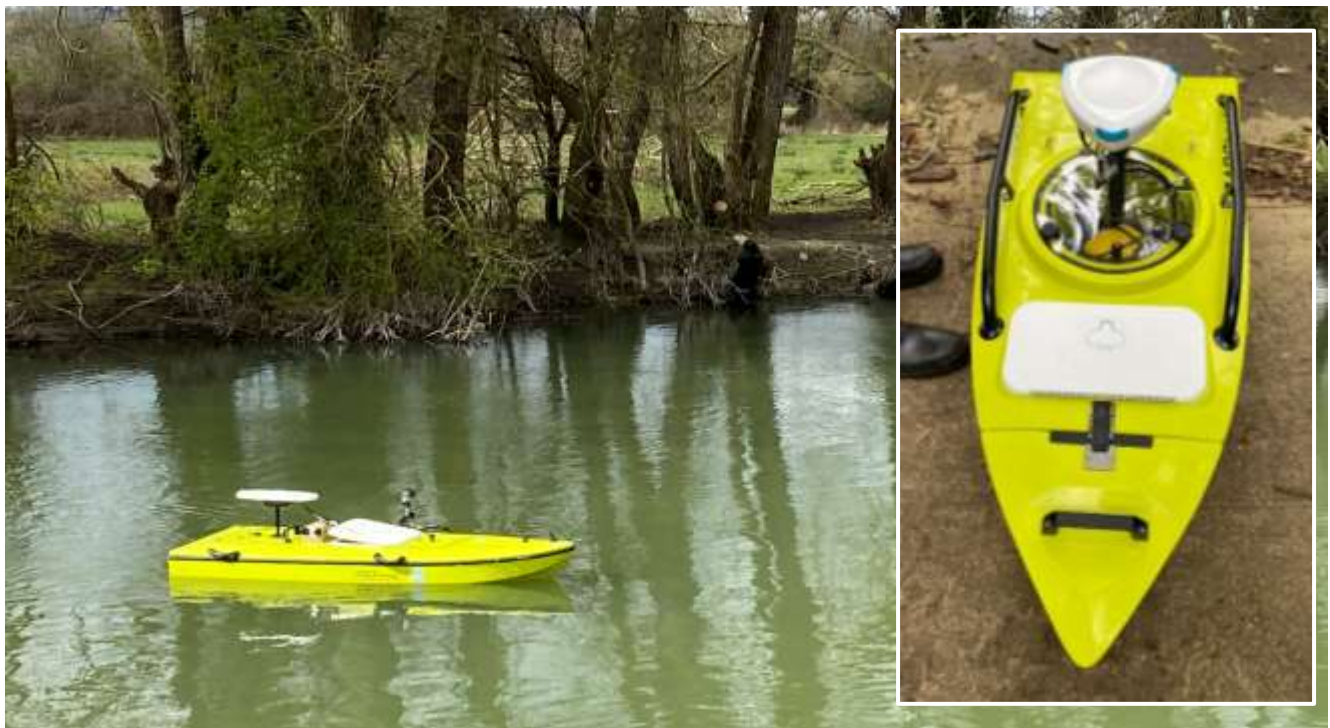
The ARCboat and (inset) ARCboatlite uncrewed river survey boats
