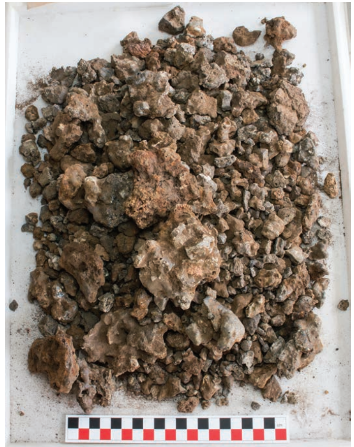
Figure 22a (above) Fuel ash and rubble slag, and figure 22b (below) smithing debris, all from the Blacksmith's workshop
