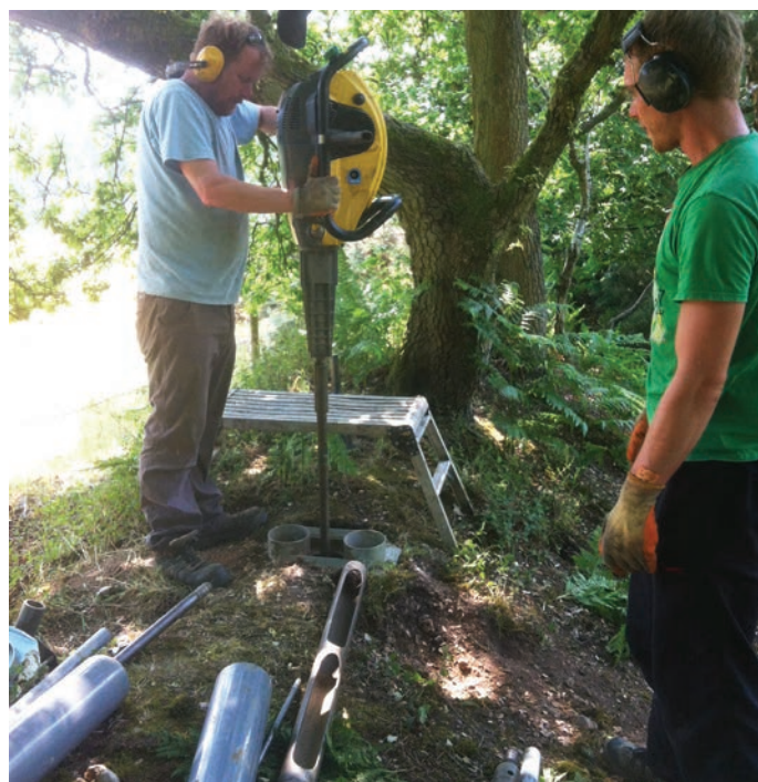
Figure 9 Coring the rampart at Pond Farm
